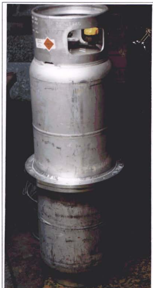
This is Brian Boland's experiment in making a take-down 15 gallon fuel tank from 2 Worthington 10 gallon tanks. the tank halves bolt together at the flanges and are sealed with a lip on one flange and an epoxy gasket compound in a groove on the other flange. The take down feature is intended to allow carrying a burner or envelope inside the tank as airline baggage.
