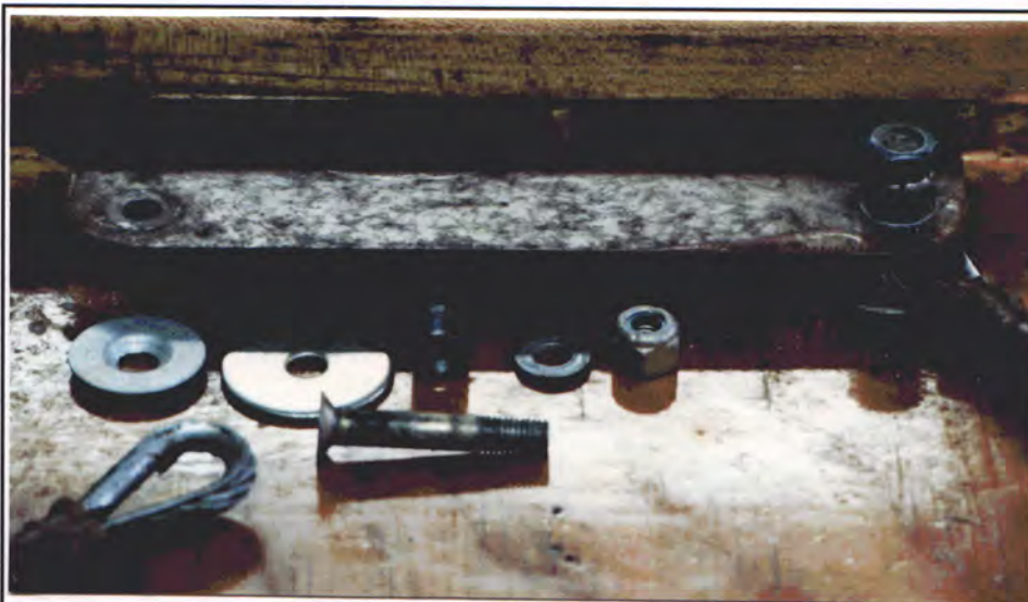
Figure 4: Here we see the steel plate, mounted between the center skids. A basket support cable is attached to each corner using an AN509 aircraft bolt. The bolt attaching the left hand cable has been taken apart to show its assembly. The right hand cable shows the normal assembled appearance.
