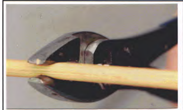
Figure 2: Here is my homebuilt reed squeezer at work. Squeezing the water-soaked reed allows it to be bent without breaking. I built my squeezer by grinding the jaws of a common pair of pliers to a rounded shape.
