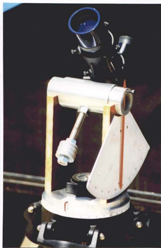
The theodolite on its tripod. Joe used phenolic sheet for his saddles. He also added a counterweight to offset the weight of the spotting scope and to provide even balance.
