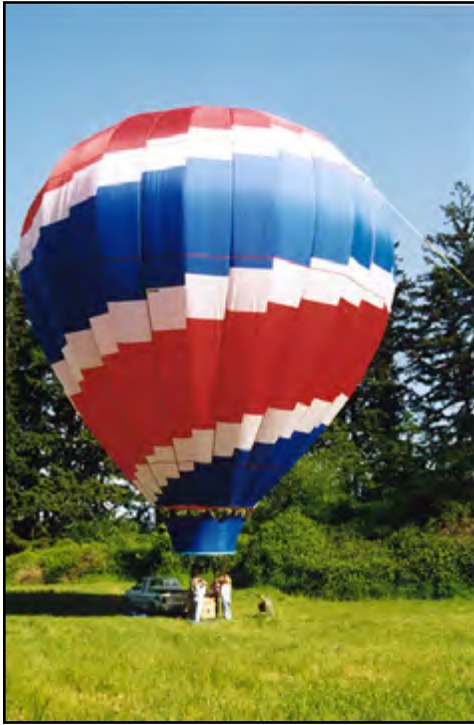
Isewbar was built in 1999. It was an S-50 design with 16 load tapes and 32 half gores. It was 54,000 cubic feet and weighed 154 pounds.
