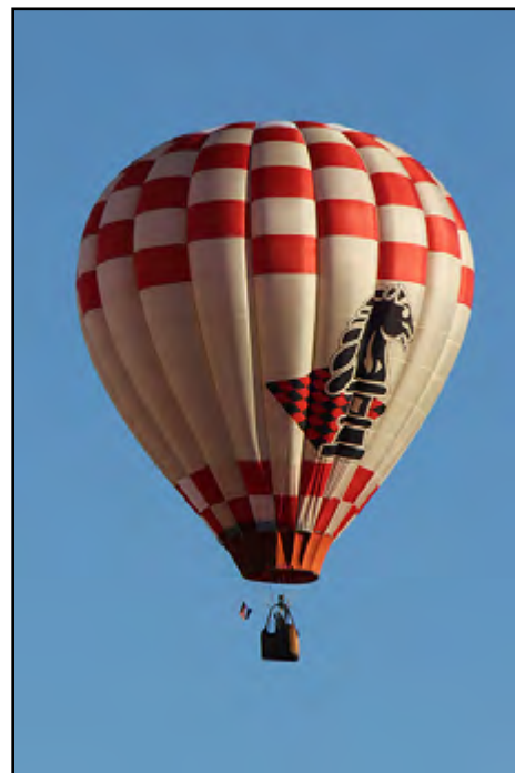
This was Checkmate, owned and operated by Tim Gale. This photo was taken on Checkmate's last flight in 2014. You can see where the mouth is sucking in because so much of the hot air is just leaking out of the top. At the end Checkmate was using over 19+ gallons of propane per hour.
