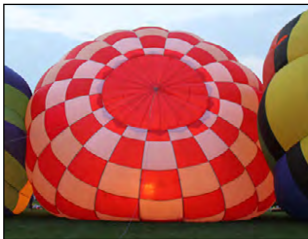
Just look at the fabric in the middle of the red bottom panel. You can see the flame right through it. Was this balloon porous? It sure was. We were sad to end her life, but it would have been unkind to try to sell her to a naive new pilot. Checkmate was sent back to the factory in North Carolina and "reskinned."
